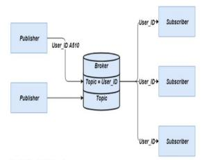
Fig. 2. The MQTT architecture.
